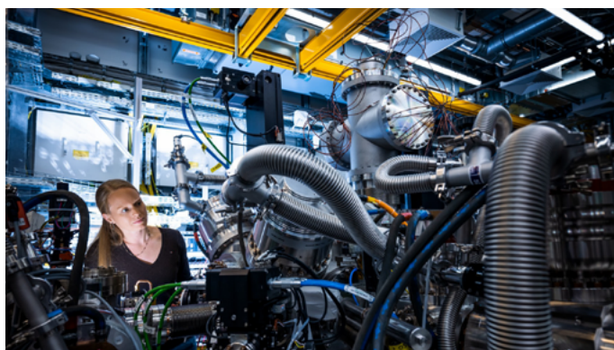
Fig. 3: Rebecca Boll at the COLTRIMS (REMI) reaction microscope of SQS instrument of European XFEL, where the experiment was carried out.
