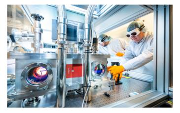
Detail view inside the TWIN amplifier of the HIBEF HI Laser at the HED instrument showing Ti:Sapphire gain medium encased in a cryogenic cooling chamber. Copyright: European XFEL / Jan Hosan
