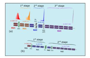
Fig. 3 FEL-2 in SR mode. Each of the radiators Rd1, Rd2 and Rd3 resonates at a low-order harmonic of the preceding one. The modulator Md1, resonant with the UV seed laser and separated from the first radiator Rd1 by the dispersive element (DS1), initiate the sequence. Seed intensity and dispersion are tuned to reach saturation at the exit of Rd1. The delay line (DL), set at low current (2.6 A), plays the role of a phase shifter ( $\Delta \phi$ ) between the two modules of Rd2.
