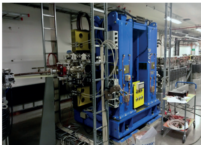
Photo: The in-vacuum undulator for the BioMAX beamline being installed at MAX IV in Lund.
