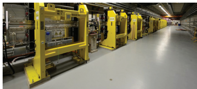
Figure 2: The 30 m long undulator in the FLASH2 line, consisting of 12 segments which produce the FEL radiation.
