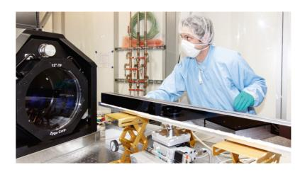
Inspecting a superflat X-ray mirror in the laboratory. The profile does not deviate from a perfect surface by more than a billionth of a metre.
