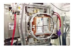
The intense pulses from XFELs require the development of new detector technologies, with spinoff to industry. The picture shows the AGIPD detector at the SPB/SFX instrument of European XFEL.
