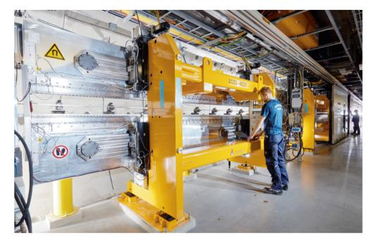
Extremely precise periodic arrangements of magnets called undulators steer electrons into a slalom course. This process causes electrons to emit light in the form of X-rays or infrared radiation. Short but intense pulses of electrons combined with long lengths of magnets result in exponential gain as the electrons continue down the magnetic structures, generating the brilliant flashes unique to FELs for use in experiments.
