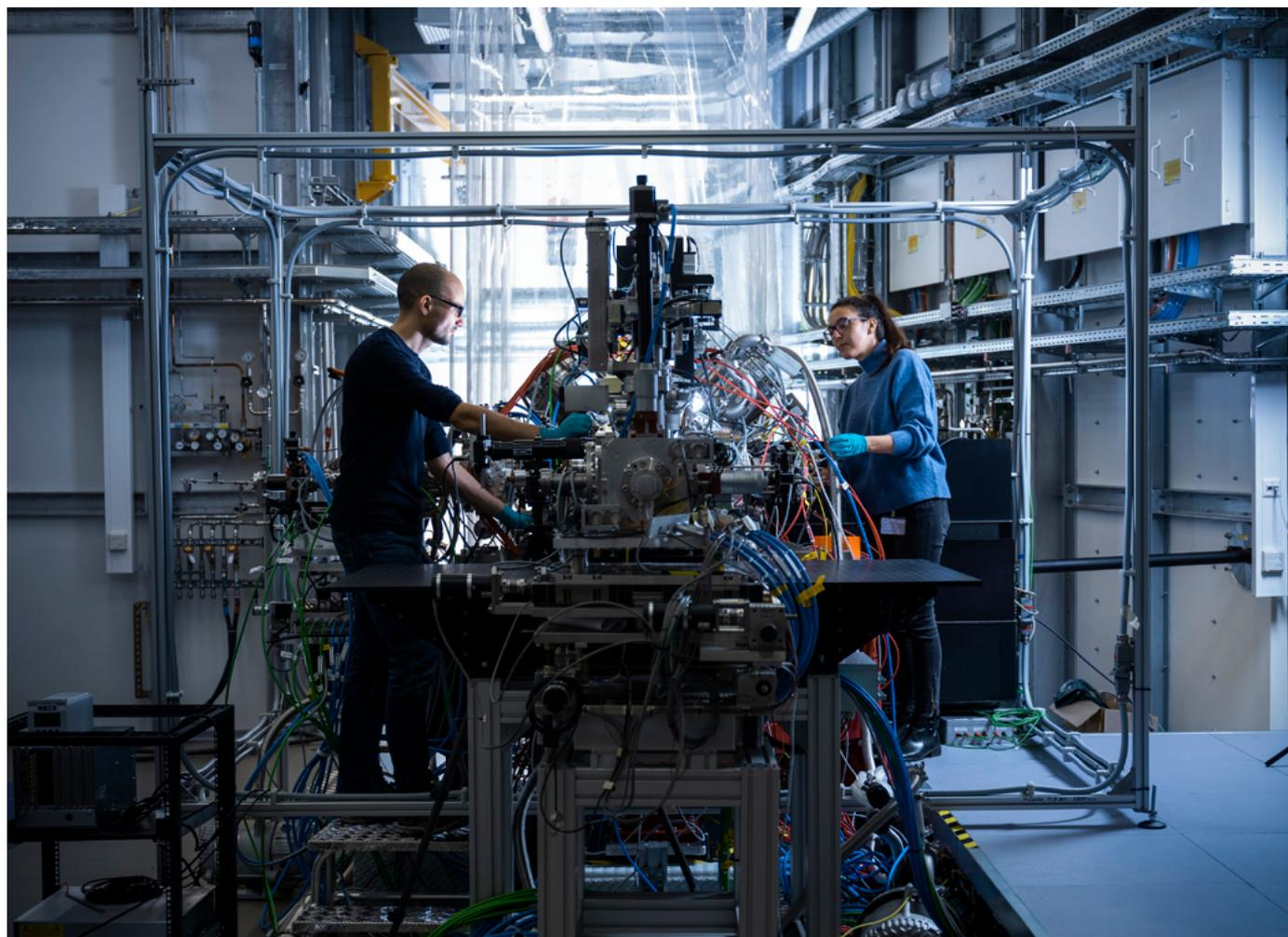
The SQS experiment station is dedicated to the study of free atoms and molecules, as well as clusters and nano-particles that consist of up to several thousands of atoms. Experiments will focus on “non-linear” multi-photon processes beyond the conventional “linear” process of absorption of just one photon, and on time-resolved investigations of the ultra-fast molecular fragmentation caused by these processes. Copyright European XFEL / Jan Hosan.
