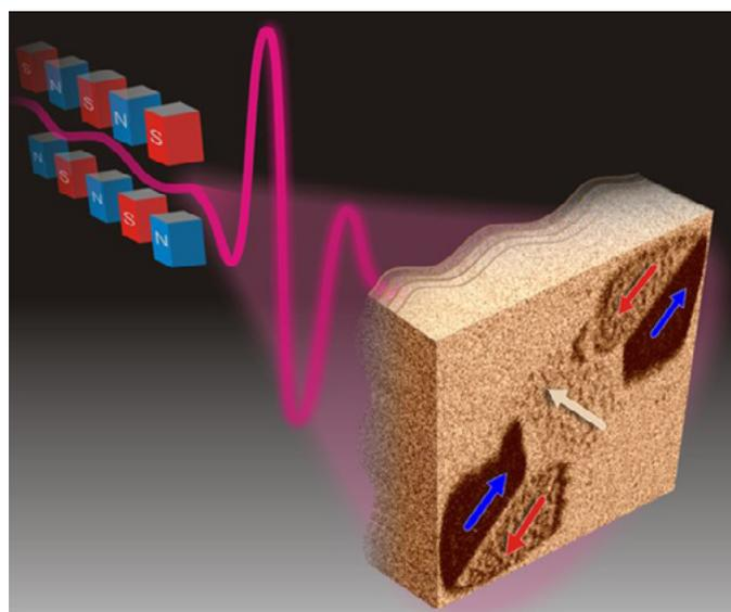
Fig 3: Four-magnetic-domain pattern switched by a FELIX pulse
