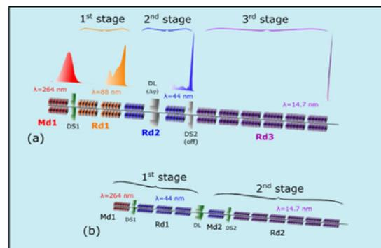
Fig. 3 FEL-2 in SR mode. Each of the radiators Rd1, Rd2 and Rd3 resonates at a low-order harmonic of the preceding one. The modulator Md1, resonant with the UV seed laser and separated from the first radiator Rd1 by the dispersive element (DS1), initiates the sequence. Seed intensity and dispersion are tuned to reach saturation at the exit of Rd1. The delay line (DL), set at low current (2.6 A), plays the role of a phase shifter ( $\Delta\phi$ ) between the two modules of Rd2.
