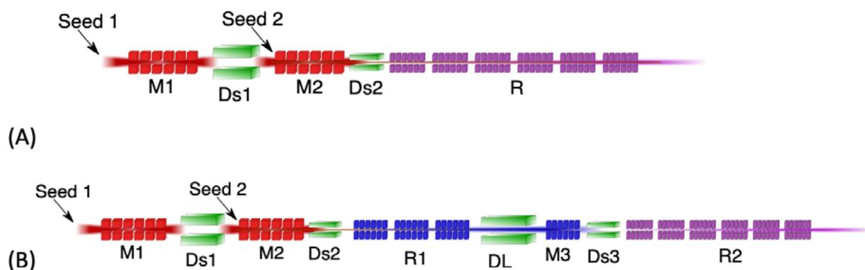
Fig 8: (A) Single stage EEHG FEL Configuration (B) Double stage cascade where the first stage is an EEHG FEL and the second stage a HGHG FEL. The second stage is seeded by the first stage in fresh-bunch injection configuration.
