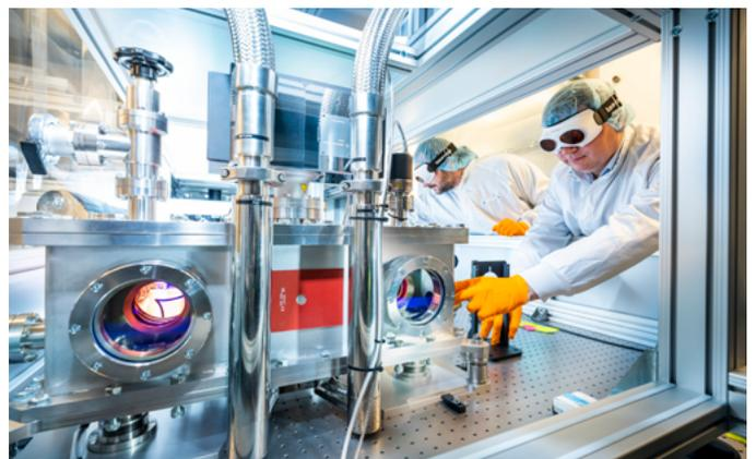
Detail view inside the TWIN amplifier of the HIBEF HI Laser at the HED instrument showing Ti:Sapphire gain medium encased in a cryogenic cooling chamber. Copyright: European XFEL / Jan Hosan
