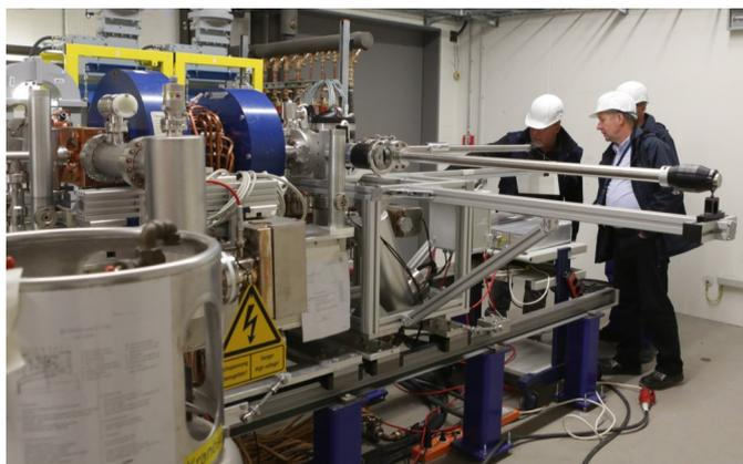
Fig. 1 - The European XFEL's electron gun, the first part of its accelerator complex, was recently installed and put through the first round of intensive tests.
