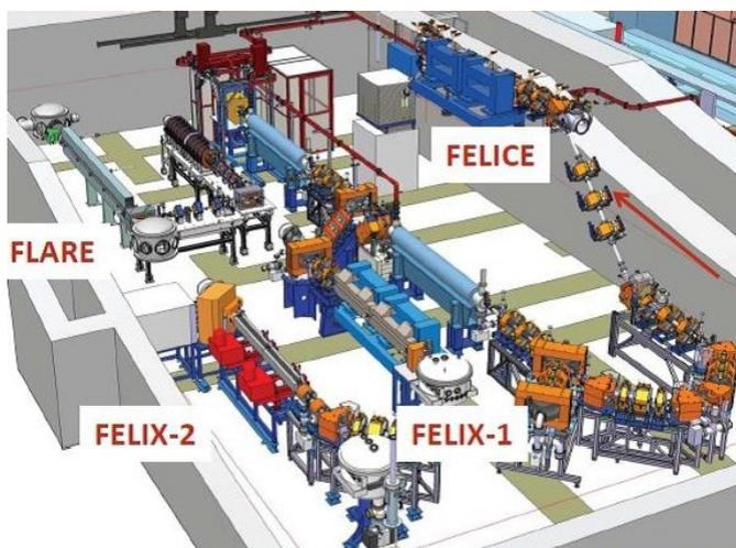
Fig. 1 - Schematic layout of the FELIX facility showing the four beam lines FLARE, FELIX-1, FELIX-2 and FELICE.
