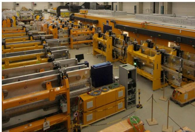
Fig. 2 - The European XFEL undulator group has successfully measured and tuned over half of the facility's light-generating undulator segments, preparing them for tunnel installation later this year.
