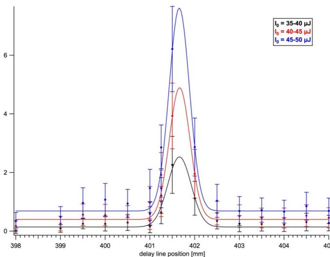
Markers: average of single-shot Xe<sup>6+</sup> signal values for FEL pulse energy falling within a given interval, as indicated by colours (black: 35-40 mJ; red: 40-45 mJ; blue 45-50 mJ). The error bars reflect the standard deviation of the values. Lines: Gaussian fit.
