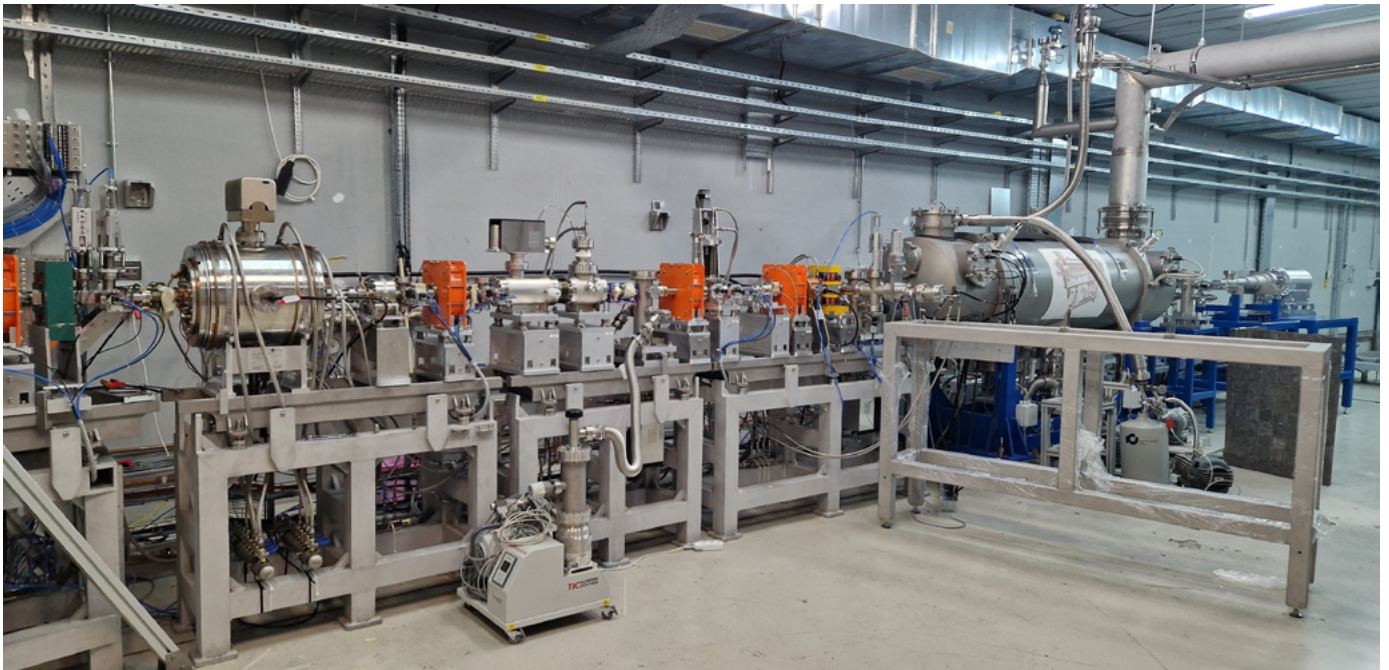
Fig. 1 Picture showing the injector beamline and the first cryomodule of TARLA electron accelerator.
