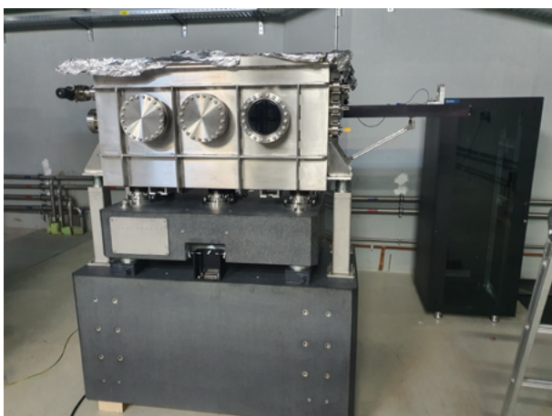
Fig. 2: M1 of the optical cavity.
